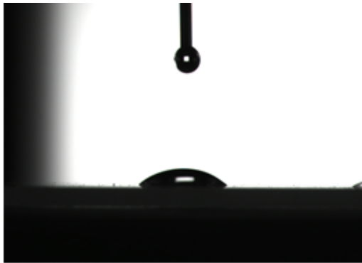
Fig.1. The contact angle of a water drop on the NCC film
